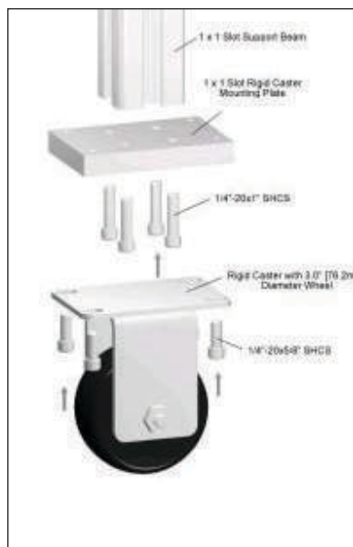
1x1 Slot Rigid Caster Assembly mounts to the end of a 1x1 Slot Support Beam to provide fixed caster mobility.
