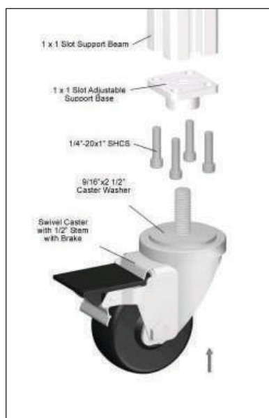
1x1 Slot Swivel Caster Assembly with Brake mounts to the end of a 1x1 Slot Support Beam to provide "breakable" swivel caster mobility.
