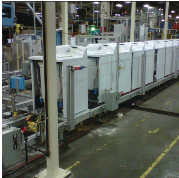
Use Tekno's own Non-synchronous Conveyor System for Palletized Product Assembly & Conveyance.
